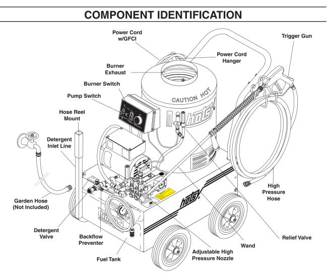
**Pump** — Delivers a specific gpm to the high pressure nozzle which develops pressure.
