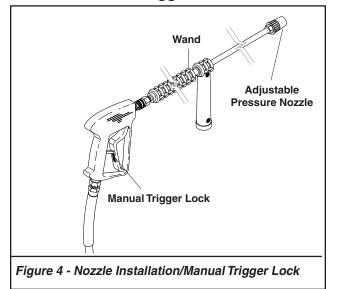
IMPORTANT: If the pressure washer has not been used for an extended period of time, remove the nozzle from the end of the wand and turn on water supply. Allow water to run from the end of the wand until clear.
