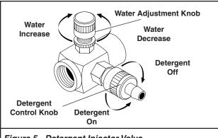
Figure 5 - Detergent Injector Valve
